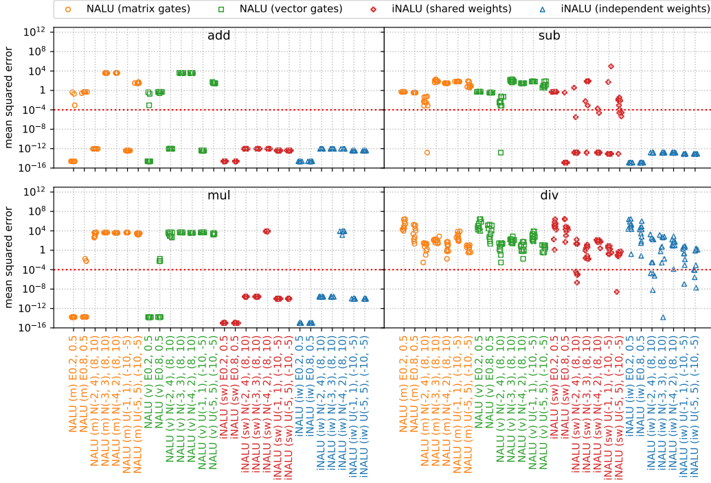
Figure 6.6: MSE for various input distributions per operation over the extrapolation test dataset of experiment 3 (simple arithmetic task). For a detailed description see Fig. 6.4.
