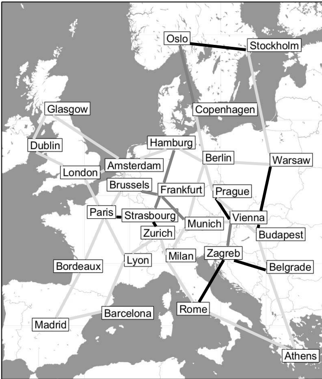
Fig. 8. The colors of the links in the Nobel network indicate their potential overload due to network failures: dark links are more likely to be overloaded; in this example, overload is defined as the probability for relative link load \rho(l) > 0.6 .
