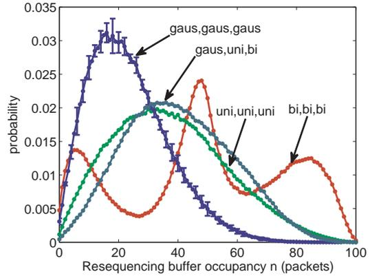
Figure 11: Buffer occupancy for three paths
