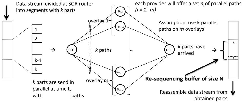
Figure 8: Transmission Mechanism
