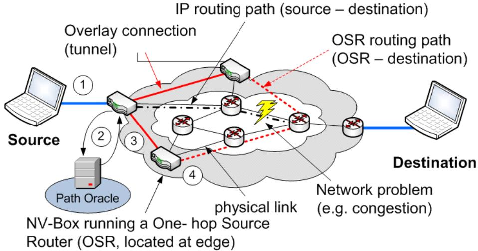
Figure 6: Routing Overlay using One-hop Source Routing
