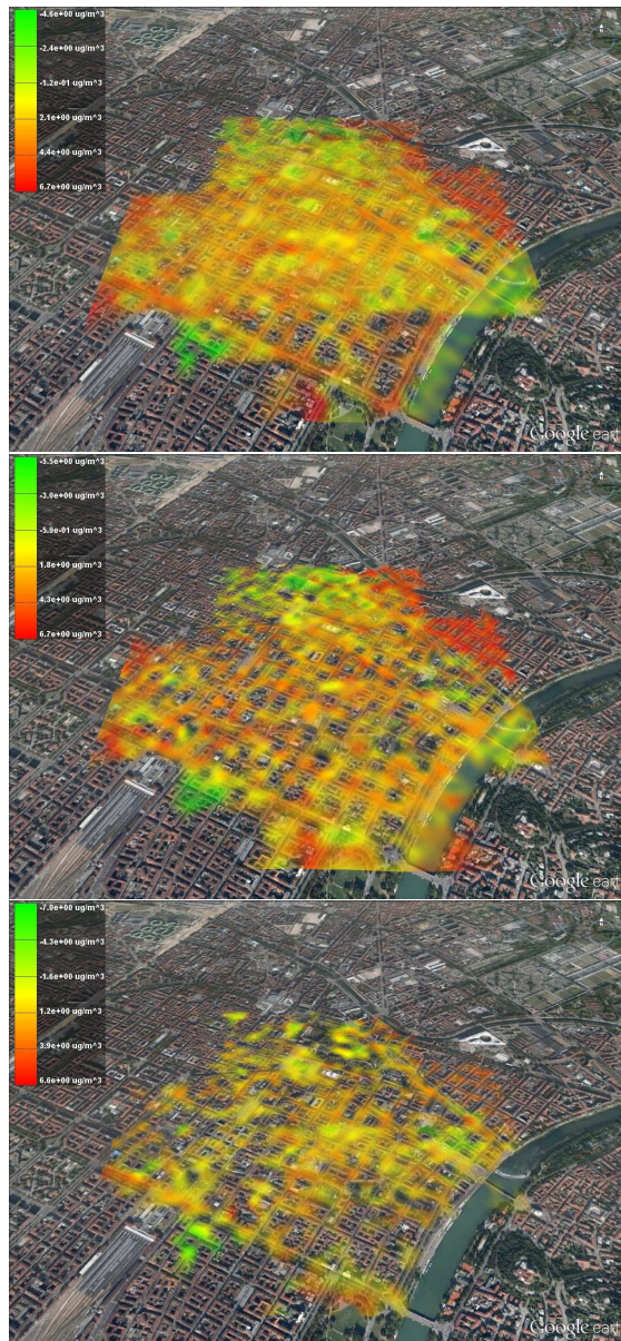
Fig. 2.13 Heat map of the APD values (difference between the web-game annotated AirPin value and the AirSquare value inferred from on field sensor box measurements) for the city of Turin. Top figure refer to phase I, the middle one to phase II, the figure at bottom to phase III. Values in the legends represent \mu\text{g}/\text{m}^3 concentration of Black Carbon. The opacity is related to the number of AirPins used in the corresponding point.
