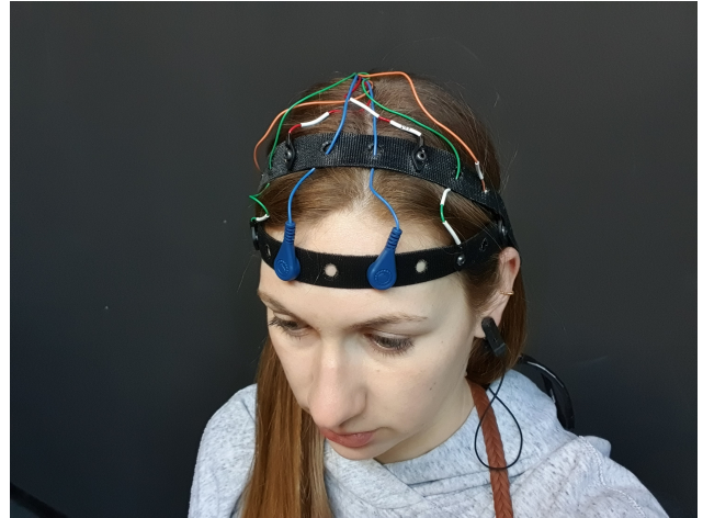
Figure 1: OpenBCI headband as worn for EEG data collection during our study.
