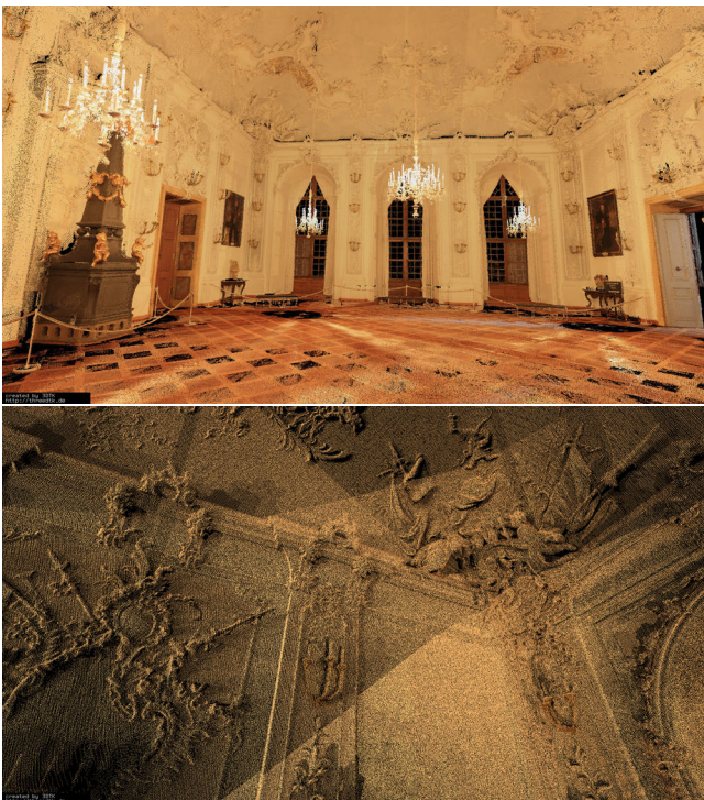
Figure 11: Reconstruction of the White Hall in the Würzburg Residence. In the close-up view the impressive stucco work is clearly visible.
