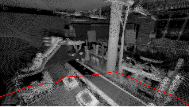
Figure 6. 3D point cloud of the laboratory. In the foreground, the trajectory is shown in red.
