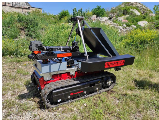
Fig. 1. RTE-robot a tracked search and rescue robot with a light robot arm, a pick-up and transport module.
