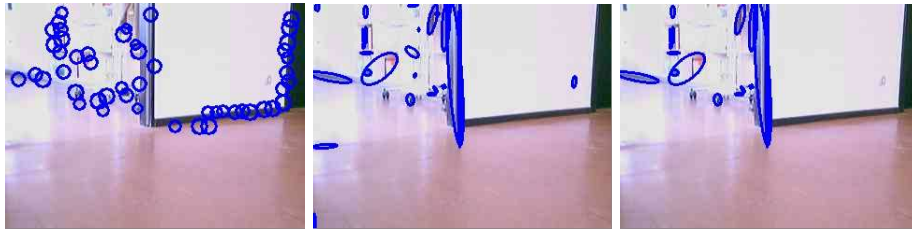
Fig. 1. Results for the saliency, the MSER and the combined saliency-MSER feature detection for the same image. The detected visual features are highlighted: Salient regions in the left, MSERs in the middle, and the overlapping regions from these both images are shown on the right image.
