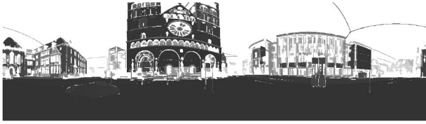
Fig. 2. Scan 0 as range-image of size 1441 \times 401 = 577841 with grayscale based on distance. The horizontal field of view (FOV) covers full 360^\circ . The vertical field of view (FOV) of the sensor is -40^\circ to +60^\circ . The façade of the St. Peter's Cathedral of Bremen is visible in the image's center.
