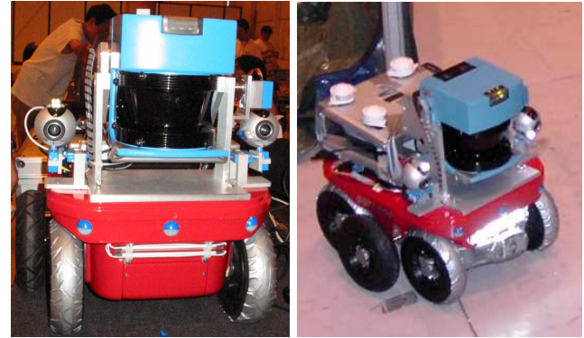
Fig. 1. The mobile robot Kurt3D equipped with the 3D laser range finder as presented at RoboCup 2004. The scanners technical basis is a SICK 2D laser range finder (LMS-200).
