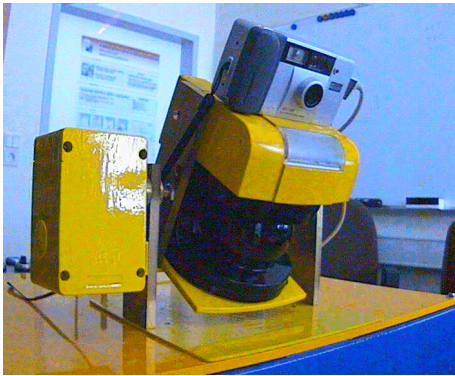
Figure 2: The 3D laser range finder. The servo is mounted at the left side. A camera on top is used to get texture images for the realistic appearances of a 3D scene.
