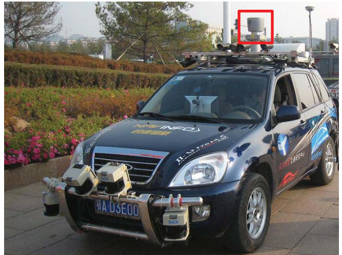
Fig. 6. The intelligent vehicle of Wuhan University:SmartV, the sensor labeled by red rectangular box is Velodyne scanner.
