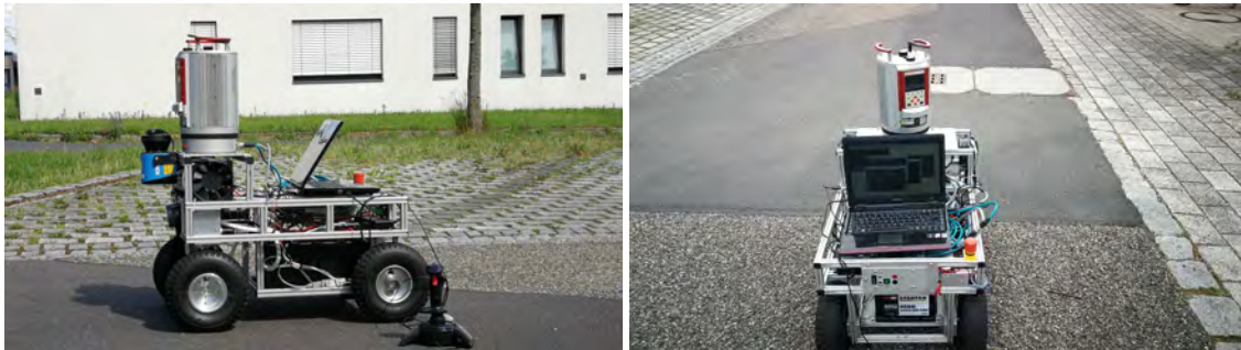
Figure 1. Images of the mobile robot mapping system.
