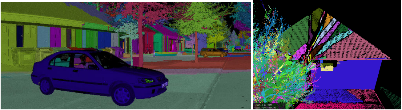
Figure 5. Results of the segmentation algorithm. Segmented car (left) and building (right). The right image is a perspective projection of a part of the 3D point cloud. Parameters used: \sigma = 2 , K = 300 , I = 100 .
