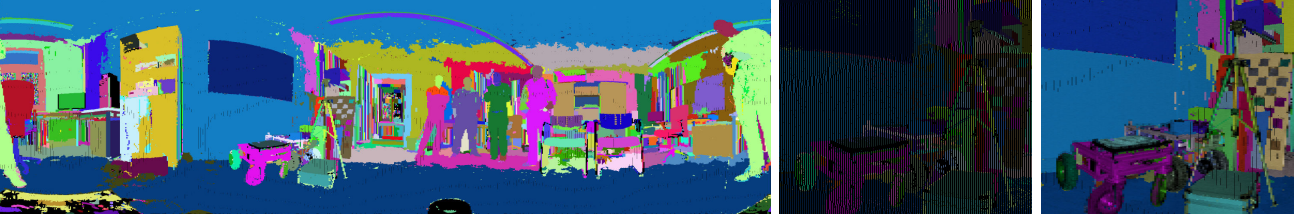
Figure 3. Segmented spherical image of the coarse data set (left), with a coarse (middle) and diluted detail (right). Parameters used: \sigma = 1 , K = 10 , I = 40 .
