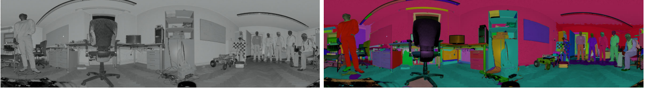
Figure 2. Spherical reflectance image (left) and its segmentation (right), using \sigma = 0.2 , K = 50 , I = 30 , and 8 nearest neighbors for every point.
