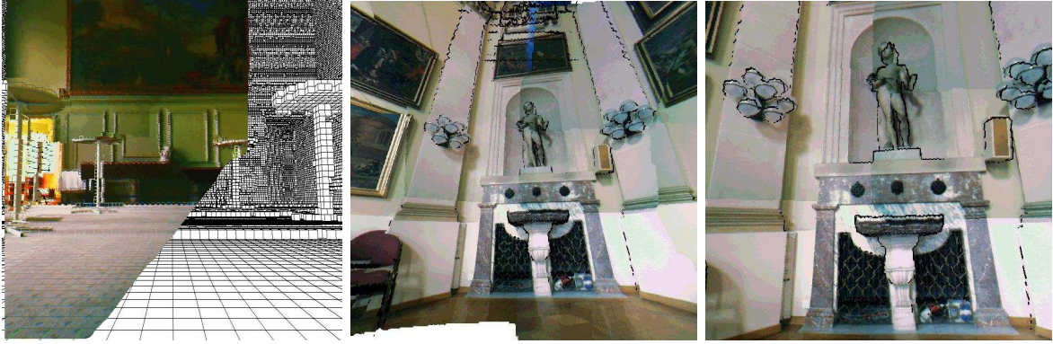
Figure 4: Left: Schematic illustration of the texture mapping process. Middle and right: Final 3D texture mapping from two different view poses of the scene given in Fig. 2, right.
