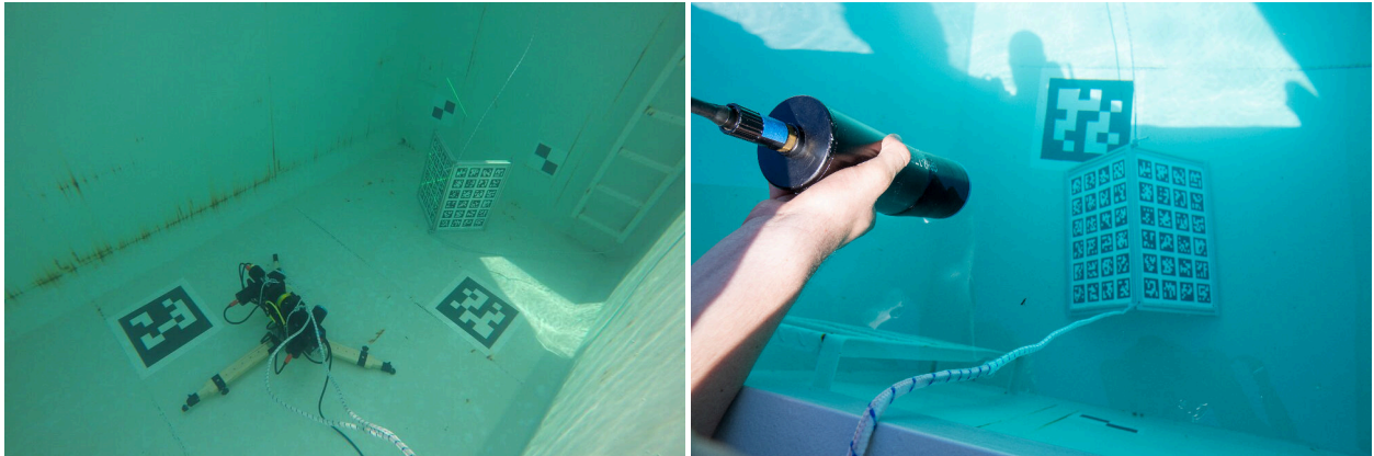
Figure 7. Left: One of the first experiments in the new test environment with our underwater 3D laser line scanner mounted on top of a tripod. Right: Experiments in the test environment for validation of refractive underwater camera models.
