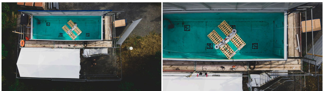
Figure 3. Top view of the water container. The placed AprilTags on the floor and an experimental setup with a raft can be seen.
