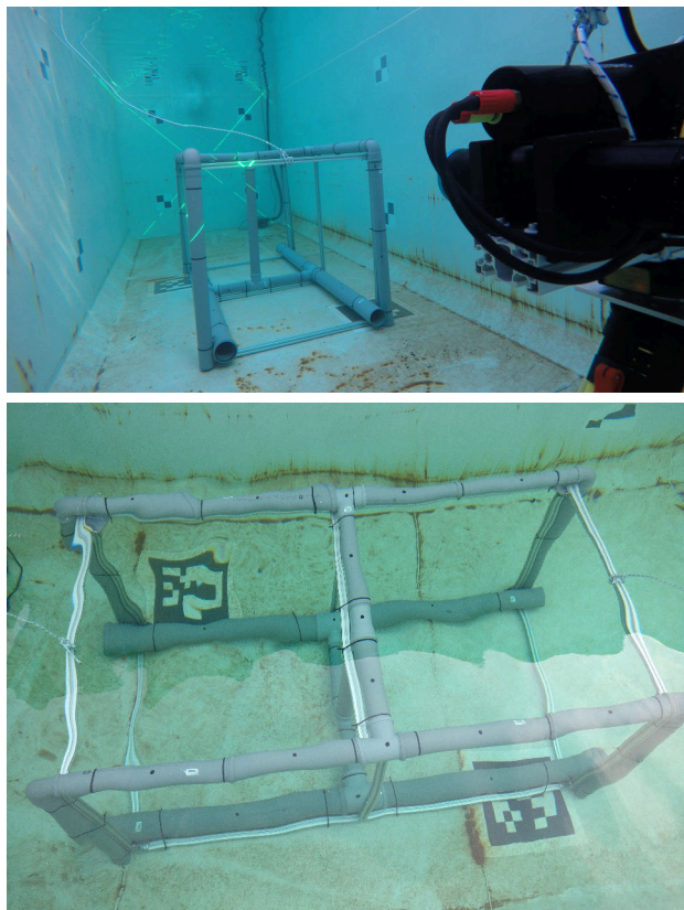
Figure 5. The first test structure placed in our water container. The size is 1 m × 1 m × 2 m and was built from item profiles and pipes.
