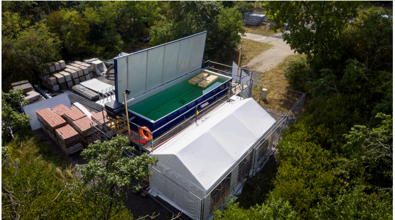
Figure 1. Overview of our test environment. The 7 m x 2.4 m x 2.4 m Roll-on/Roll-off container filled up with around 40 000 l of water, a tent to have a dry working place and the scaffolding around the container are visible.
