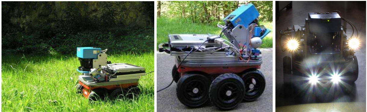
Figure 1: The mobile robot Kurt3D equipped with the 3D laser range finder. The 3D scanner's technical basis is a SICK 2D laser range finder (LMS-200). The robot is completely independent from external light.
