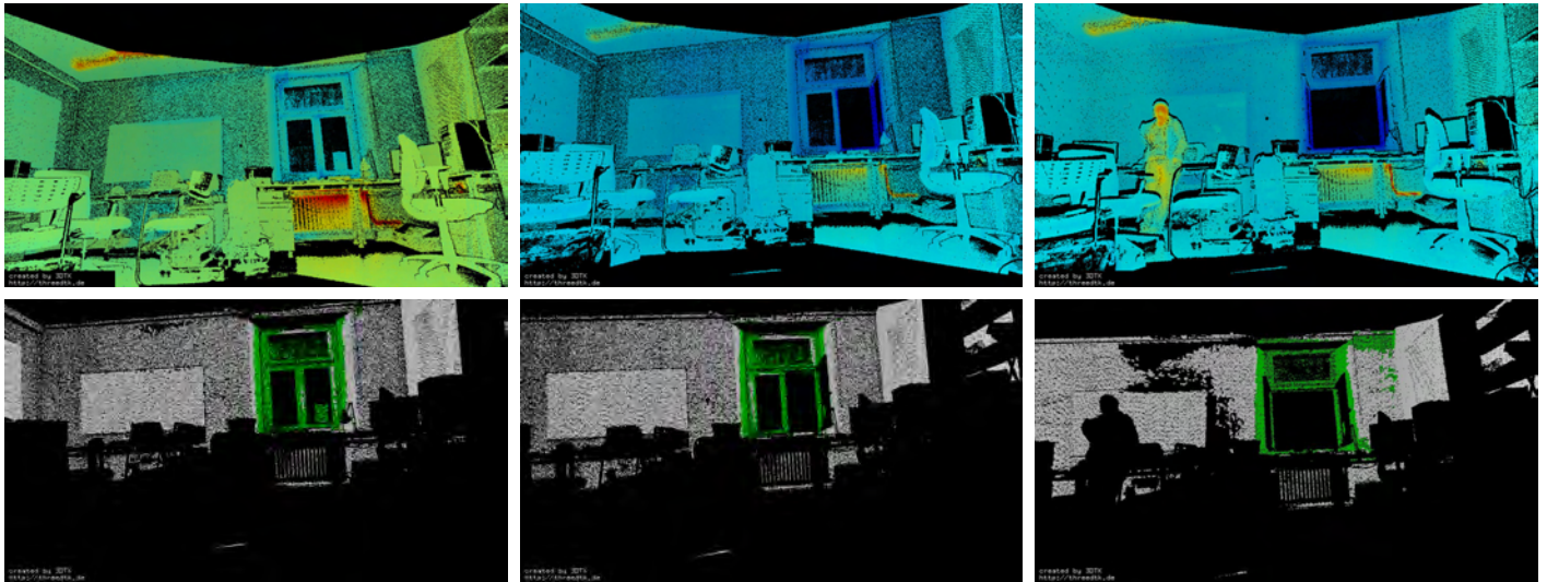
Fig. 7: Top: Three original thermal 3D point clouds with temperature values. Bottom: The detected windows under different circumstances, i.e., closed, semi-open, and fully open are shown in green.
