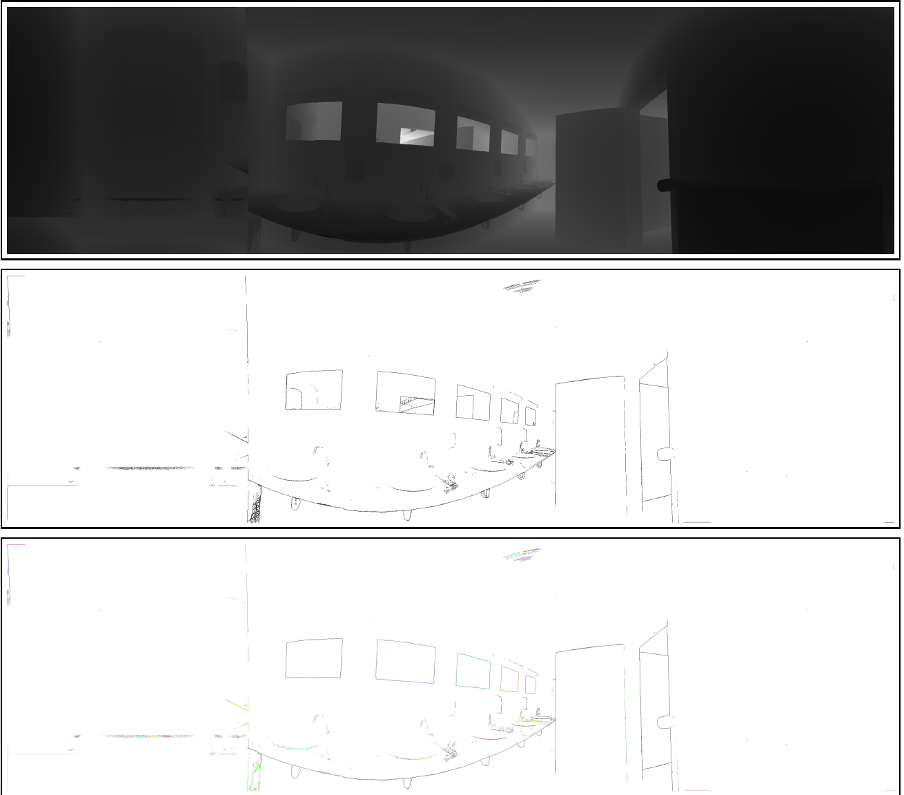
Figure 3: Top: Range image of scanned bathroom environment with five mirrors of same size and resolution of 3600 \times 1000 . Middle: Corresponding jump edge image with a threshold of 0.1 m. Bottom: Extracted 2D contours of picture above.
