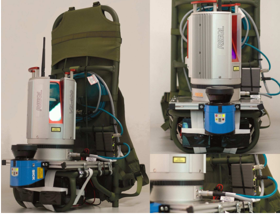
Figure 2. Images of the backpack system. Left: Side view with all of its sensors and equipment. Right: Detailed view of the SICK and the switch.
