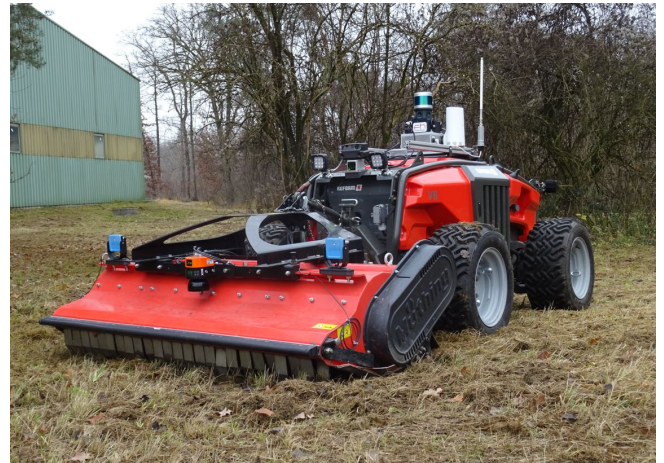
Fig. 1: Carrier platform with attachment and automation kit
