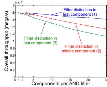
**Fig. 7.** Impact of an early non-match decision for AND-filters on the message throughput depending on the filter complexity for a replication grade of  $r = 1$ .
