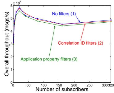
**Fig. 5.** Impact of filter activation and the number of subscribers on the message throughput.
