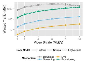
Fig. 5: Influence of Bitrate, Download Mechanism and User Model on Wasted Traffic
