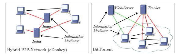
Figure 4: Hybrid P2P overlay topologies
