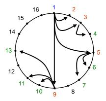
Figure 8: Model of the search in a P2P network
