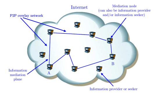
Figure 2: A P2P overlay network used as information mediator
