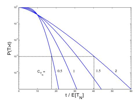
Figure 11: Distribution of the search delay for different values of  $c_{T_N}$
