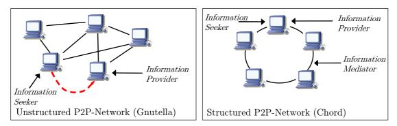
Figure 3: Unstructured and structured P2P overlay topologies
