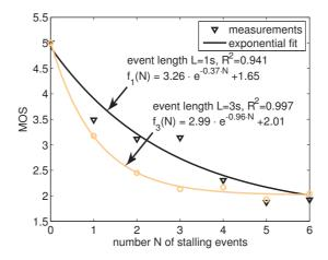
Figure 11: Mapping functions of stalling parameters to mean opinion scores
