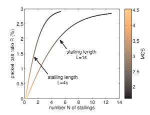
Figure 13: MOS color plot wrt. stalling frequency (TCP) and packet loss ratio (UDP)
