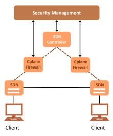
Figure 4: Control plane firewall implemented as southbound connection proxy.
