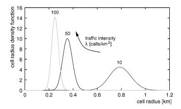
Figure 14. Density function of the cell radius for different spatial traffic intensities.
