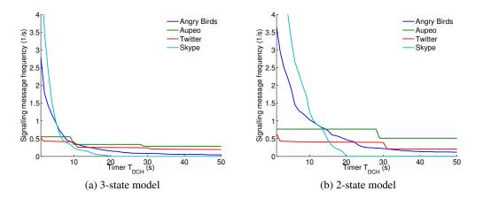
Figure 4: Signalling message frequency for varying  $T_{DCH}$  timers.
