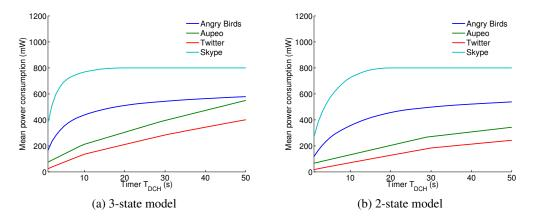
Figure 5: Power drain for varying *T*<sub>DCH</sub> timers.
