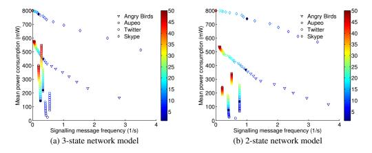
Figure 6: Influence of manipulating  $T_{DCH}$  timer on signalling message frequency and power consumption. Filled marker highlights  $T_{DCH} = 11$  seconds.
