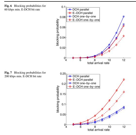
service load factor, E-DCH users may still connect to the system whereas DCH users are already blocked. The comparison of the parallel (solid lines) with the one-by-one scheduling case (dashed lines) shows that the throughput gain of the one-by-one users leads to lower blocking probabilities, and also to a higher difference between DCH and E-DCH users.
