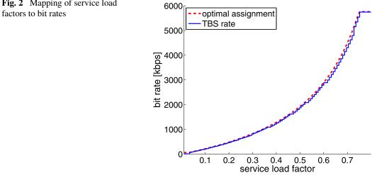
a TTI of 2 ms, the information bit rate per second follows as  $R_{i,E}^{I} = TBS_{i} \cdot 500$ , where  $i = 1, ..., |\mathcal{TBS}|$  indicates the index of the TBS. We further define  $R_{0,E}^{I} = 0$ . With this interpretation we can map the E-DCH bit rate to a service load factor according to (6) as
