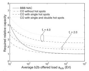
(a) Influence of the b2b offered load  $a_{b2b}$  in Labnet03 for hot spot factors of  $f_h = 2$  and 4.
