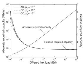
Figure 1: Impact of the offered load on the absolute and relative required capacity of a single link for various dimensioning methods.
