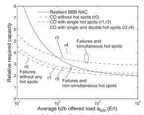
(a) Influence of the b2b offered load  $a_{b2b}$  in Labnet03 for a hot spot factor of  $f_h = 2$ .
