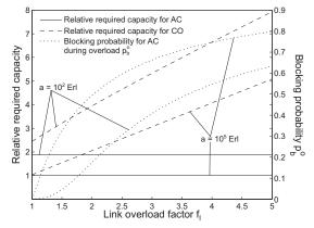
Figure 4: Impact of the overload factor  $f_l$  on the required capacity and the blocked traffic of a single link for  $a = 10^2$  and  $10^5$  Erlang.
