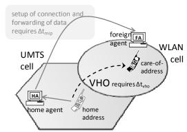
Figure 3. Introduced time delays  $\Delta t_{vho}$  and  $\Delta t_{mip}$  due to vertical handover and mobile IP techniques to overcome re-queuing in P2P system, respectively
