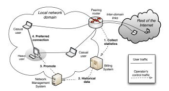
Figure 1: Example of highly active peer promotion from the perspective of a single network operator.
