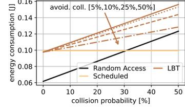
Figure 5: Energy consumption for variable collision probabilities (Sc 3).
