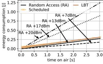
Figure 3: Energy consumption for channel access approaches (Sc 1).
