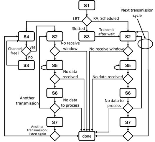
Figure 2: LoRaWAN channel access process diagram.
