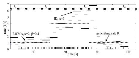
Figure 7: DI and EWMA-DI in comparison.
