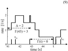
Figure 5: Rate measurement based on moving average with  $\Delta = 2$ .
