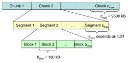
Fig. 2. Structure of a file on eDonkey application layer
