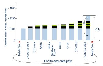
Fig. 1. Delay of an IP packet on the path between two terminals
