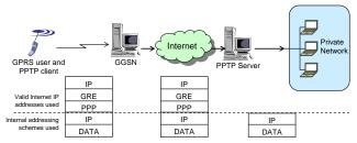
Fig. 2. Connecting a PPTP client to the private network
