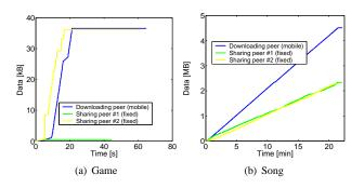
Fig. 9. Multiple source download from two peers with fixed access
