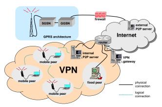
Fig. 3. Network architecture for a mobile P2P file-sharing service
