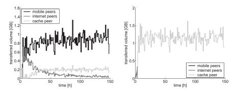
Fig. 6. Uploaded data volume of mobile and Internet peers and of the cache peer
