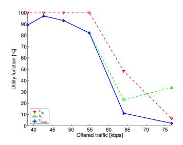
**Fig. 4.** Utility functions versus  $U_{\text{Netw}}$ ,  $U_m$  and  $U_c$  versus offered traffic  $o_A$  in the UMTS uplink case.
