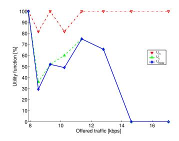
**Fig. 5.** Utility functions versus  $U_{\text{Netw}}$ ,  $U_m$  and  $U_c$  versus offered traffic  $o_A$  in the GPRS uplink case.
