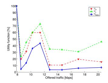
**Fig. 3.** Utility functions  $U_{\text{Netw}}$ ,  $U_m$  and  $U_c$  versus offered traffic  $o_A$  in the GPRS downlink case.
