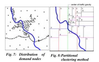
extension of  $15 \text{km} \times 15 \text{km}$ . Fig. 6 shows the traffic intensity distribution in this area, characterized by the traffic matrix: dark squares represent an expected high demand for mobile service, bright values correspond to a low teletraffic intensity. Fig. 7 depicts a simplified result of the demand discretization. The demand nodes are dense in the city center and on highways, whereas they are sparse in rural areas.
