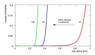
Fig. 14: Impact on customer-BTS distance on outage probability
