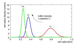
Fig. 6: Density function of the cell radius for different spatial traffic intensity
