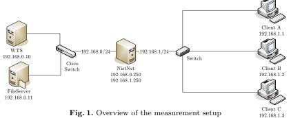
Fig. 1. Overview of the measurement setup
