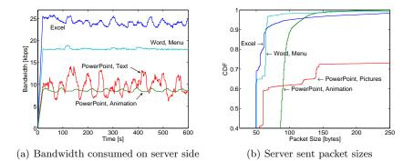
Fig. 4. Traffic characteristics varying with applications
