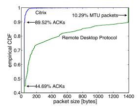
Fig. 5. Empirical CDF of the packet sizes sent during the Excel chart test.
