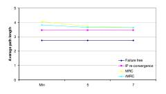
Fig. 7. Mean path length as function of the number of topologies. All networks have 32 nodes and 64 links. "Min" means the minimal number of backup topologies achieved by our algorithm for the given input topology; typically 3 or 4.
