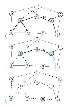
Fig. 1. Fault-tolerant multi-topology routing, sample backup configuration in MRC (a) and relaxed MRC (b, c). Nodes 3, 4 and 5 are isolated. Link 3-4, 3-6, 3-7, 4-5 and 5-9 are isolated and do not carry any traffic in MRC (a). In (b), only links 3-4 and 4-5 are isolated. The rMRC backup topology where node 6 is isolated is shown in (c).
