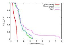
Fig. 9. Load distribution on Geant links.
