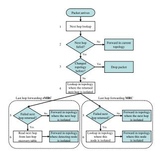
Fig. 2. rMRC and MRC forwarding. It illustrates the difference in how they solve last hop failures (steps 5-6).
