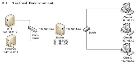
Fig. 1. Overview of the measurement setup
