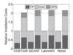
Fig. 3. Installation costs split by the considered components in the network instances
