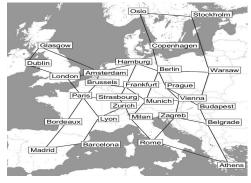
(d) Nobel: 25 nodes and 41 bi-directional links [22].Fig. 2. THE CONSIDERED NETWORK INSTANCES
