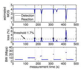
Fig. 11. Improvements by the Traffic Controller in the out-band scenario
