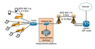
Fig. 1. Measurement setup
