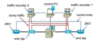
Fig. 6. Testbed setup for IP SLA measurements
