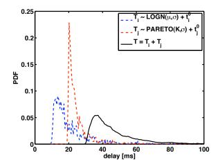
Fig. 5. Example for the estimation of delay of two individual network segments
