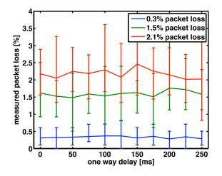
Fig. 10. Measured loss rate for increasing delay
