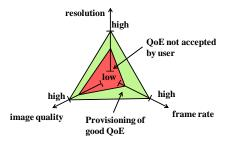
Fig. 1. Acceptable area of QoE control knob settings
