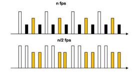
Fig. 3. Video with different frame rates
