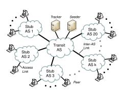
Fig. 1. Simulated network topology consisting one transit AS and n = 20 stub ASes. Every stub AS  $k \in \{1, ..., n\}$  is connected to the transit AS which only forwards the traffic.
