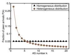
Fig. 2. Fraction of peer arrivals with respect to the AS number k. In the heterogeneous case the fraction of peer arrivals decreases for larger values of k (cf. Eq. (1)) while it is constant in the homogeneous case.
